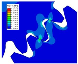
Fig. 5. Distribution of reduced stress for two-pair teeth mating of the gear with pinion no1
