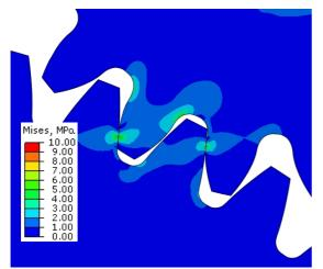
Fig. 6. Distribution of reduced stress for two-pair teeth mating of the gear with pinion no2
