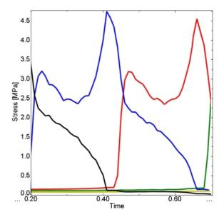
Fig. 7. The pattern of bending stress  $\sigma_z$  at roots of selected teeth of the gear
