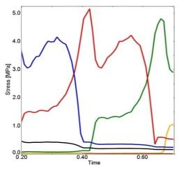
Fig. 9. The pattern of bending stress variation  $\sigma_z$  at roots of subsequent mating teeth of pinion no 2
